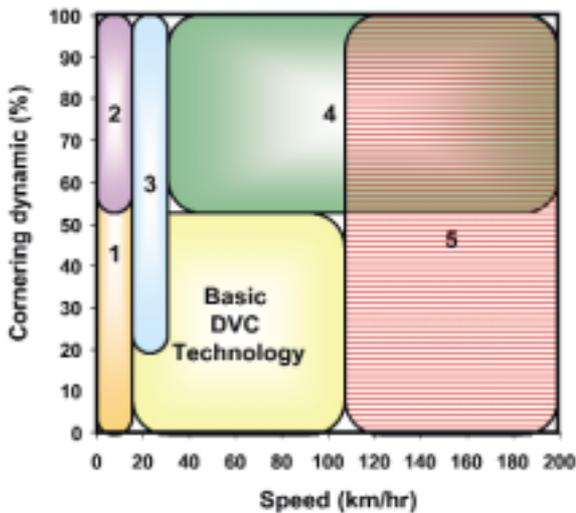
Figure 5: The additional technologies for widening the drivability envelope. This drivability area is schematically represented as a combination of driving speed and cornering dynamics. For example, bottom right represents highway driving, and top left represents dynamic cornering in the city.
