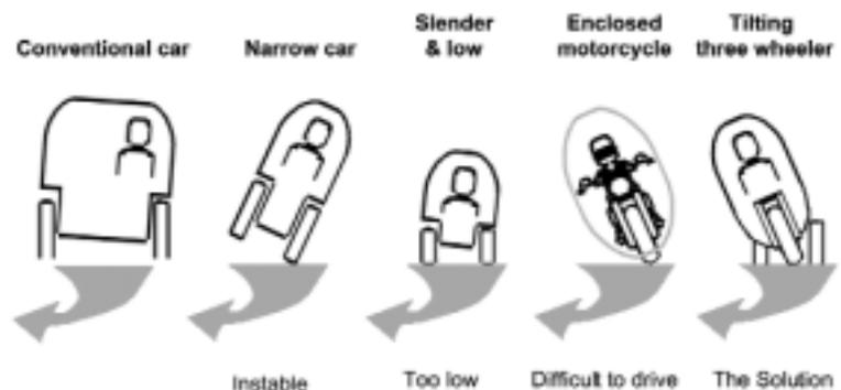
Figure 2: Tilting when cornering is the best option.
