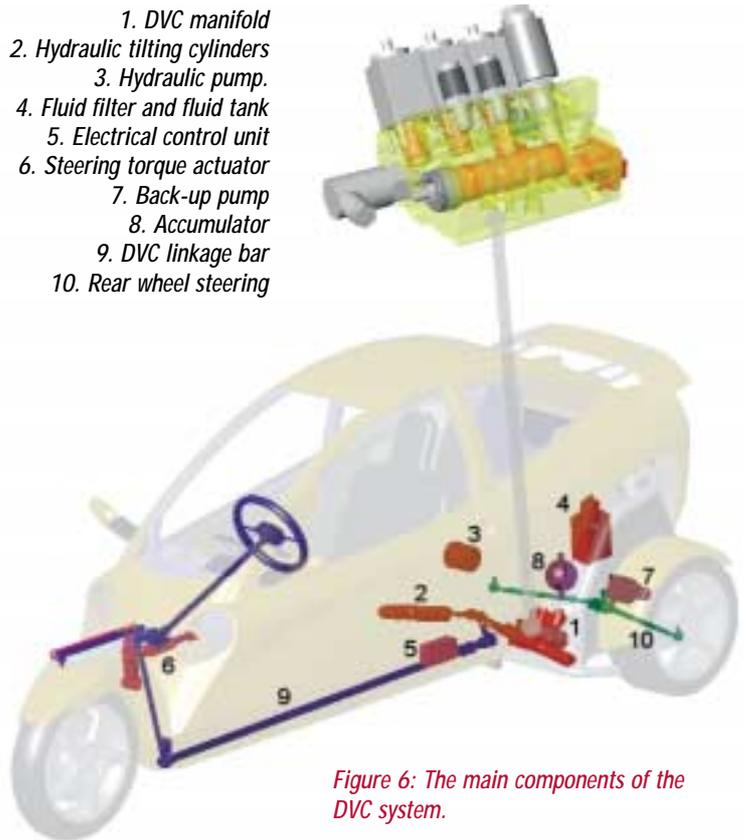
Figure 6: The main components of the DVC system.
